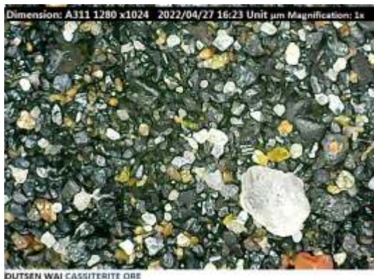
Plate 3: Micrograph of Dutshen Wei Cassiterite ore Sample under plane polarized light ( \times 1000 )
