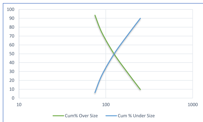
Figure 4: Sieve analysis graph indicating 80% passing
