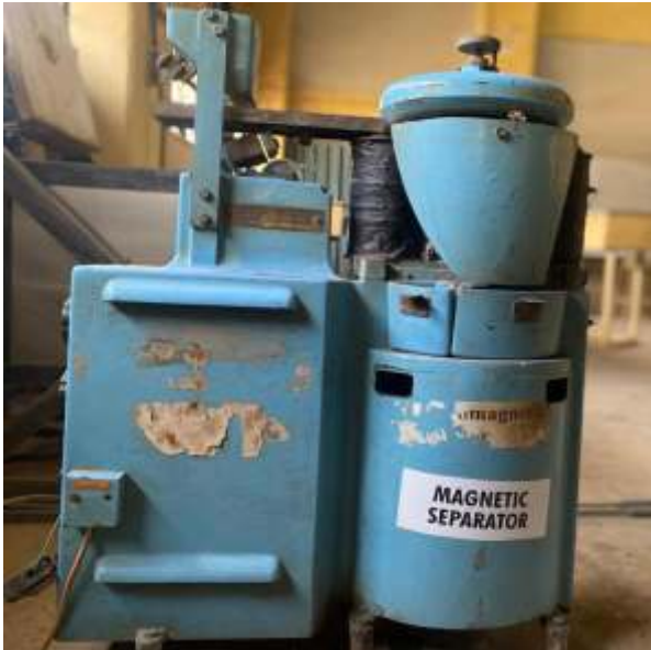
Figure 8: The Activated Electromagnetic Separator
