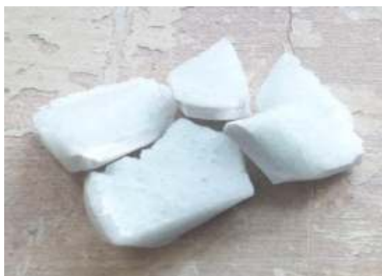
Figure 2. Melt Produced from Processed Silica Sand Sample
