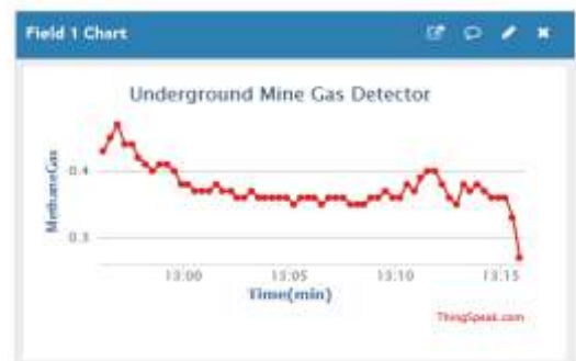
Figure 8: Graphical model showing Methane gas feed (0.48 ppm)
