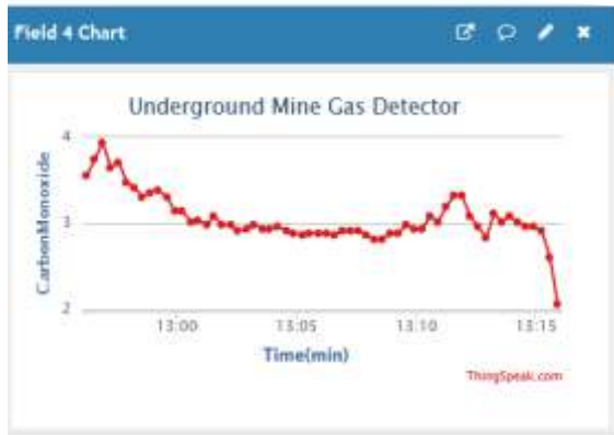
Figure 4.3: Graphical Model showing Carbon Monoxide gas feed (4ppm)
