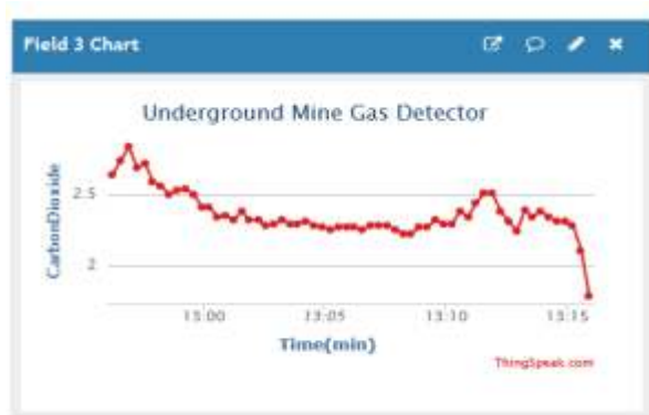
Figure 4.4: Graphical Model showing Carbon Dioxide gas feed (2.8 ppm)
