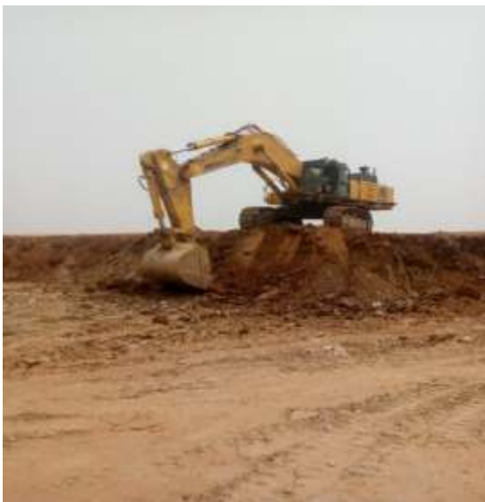
Fig 1: Komatsu Excavator use for overburden scooping.
