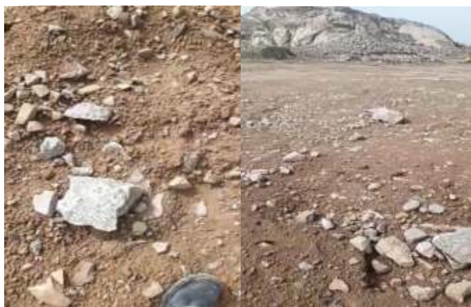
Fig. 3.4: Fly Rock at Zeberced limited quarry at a distance of 1km from where the blasting took place
